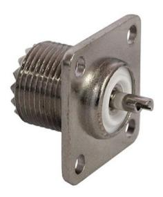
This is the first thing you will need to build a Quarter (1/4) Wave Ground Plane antenna. It's called an SO-239. You can pick one up at Radio Shack or your favorite Electronic Supply. You might want to get a couple of them just in case you damage it on the first try. I don't recommend soldering the ground plane radials. Instead use 4-40 bolts (Home Depot) and the 4-40 nuts to fit them.
