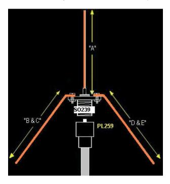
You don't have to strip all the Romex if you don't want to for the B&C/D&E. But you should have no insulation on the areas where you connect the wires to the SO239. I used the already bare ground wire for my Radiator (A).
